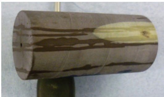
Figure 3: Hydraulic fractures produced in a laboratory specimen of slate. Fractures parallel to the length of the cylindrical sample (25 mm diameter) are oozing oil. The fractures were produced by injecting pressurised hydraulic oil into the specimen until it split apart on several fracture planes.
