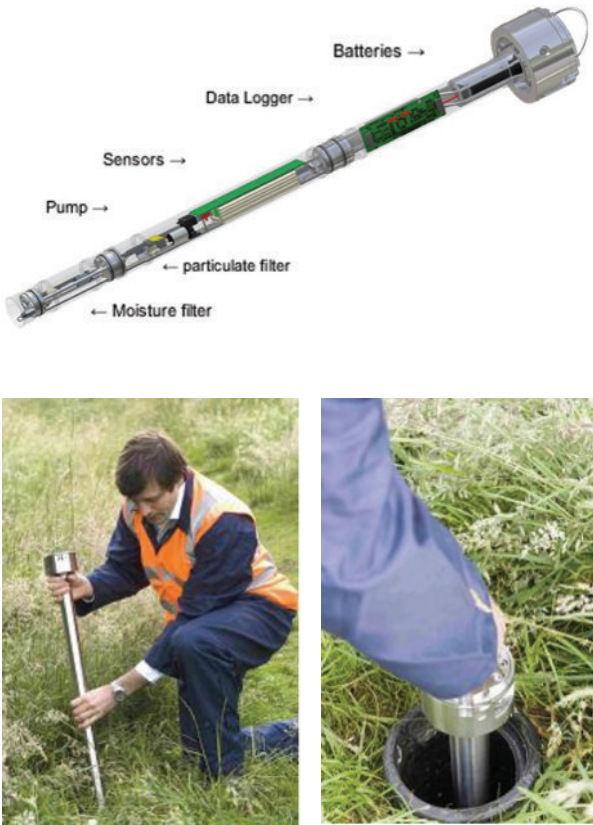
Figure 5: Cutaway diagram showing major components of Gasclam and method of installation.
