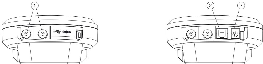
① Banana plugs for transmitter connection | ② USB 2.0 port | ③ Battery charger connection
