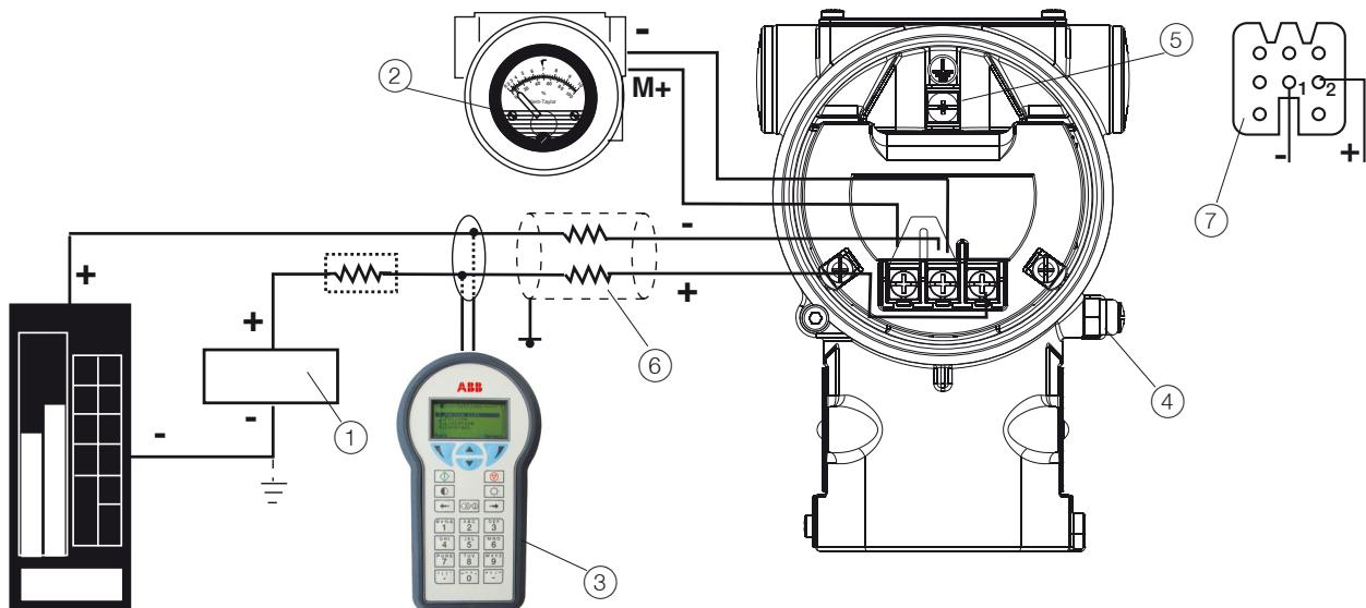
① Power source | ② Remote indicator | ③ Handheld communicator | ④ External ground termination point | ⑤ Internal ground termination point |
